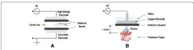
**Figure 2** . Diagram of a Dielectric Barrier Discharge and a Floating Electrode Dielectric Barrier Discharge. A presents the formation of Plasma by the Dielectric Barrier Discharge (DBD) and **B** presents the Floating Electrode Dielectric Barrier Discharge (FE-DBD).
