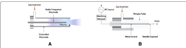
**Figure 3** .Diagram of a Atmospheric Pressure Plasma Jet and a Plasma Needle. A presents a schematic of the APPJ created by Schütze et al in 1992 and **B** presents a schematic of the plasma needle created by Stoffels et al in 2004.
